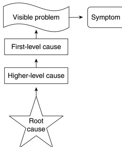
FIGURE 1. ROOT CAUSE VISUALIZED<sup>86</sup>
